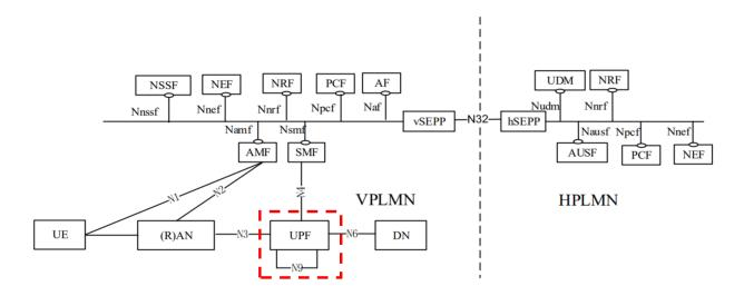
Figure 1: Roaming 5G System architecture- local breakout scenario in service-based interface.
